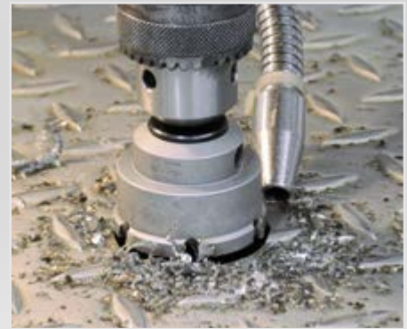
Drilling in checker sheet
