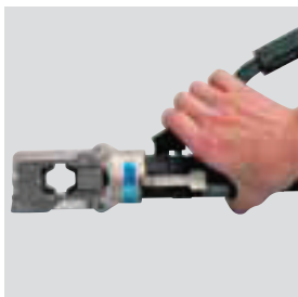
EP-50 (One hand operation to hold connector)
